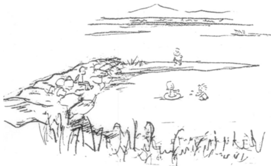
Figure 5.23 The image of belt deposition at dike toe (pattern G in Fig. 5.21). The belt creates a safe zone for water play and forms visual division that makes the broad water surface more friendly and varied
