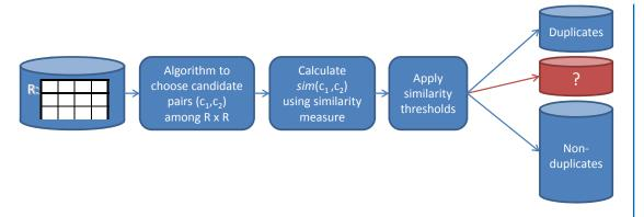
Figure 1.1: A prototypical duplicate detection process
