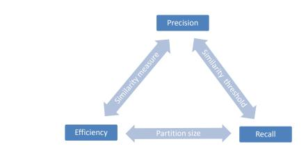
Figure 5.5: Tradeoffs between precision, recall and efficiency
