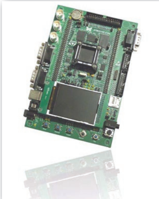
Figure 7. An evaluation board for the STM32F103MCU from STMicroelectronics, a leading microprocessor manufacturer
