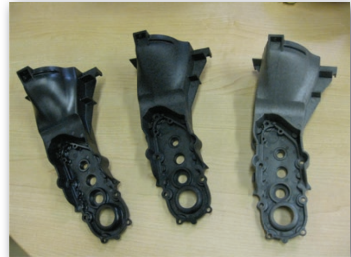
Figure 15. Testing three materials for an injection-molded plastic part from a brand new mold
