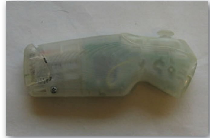
Figure 11. A typical example of a Phase 1 engineering prototype. The fully assembled prototype represents production intent part design. Custom parts are typically produced using rapid prototyping techniques.
