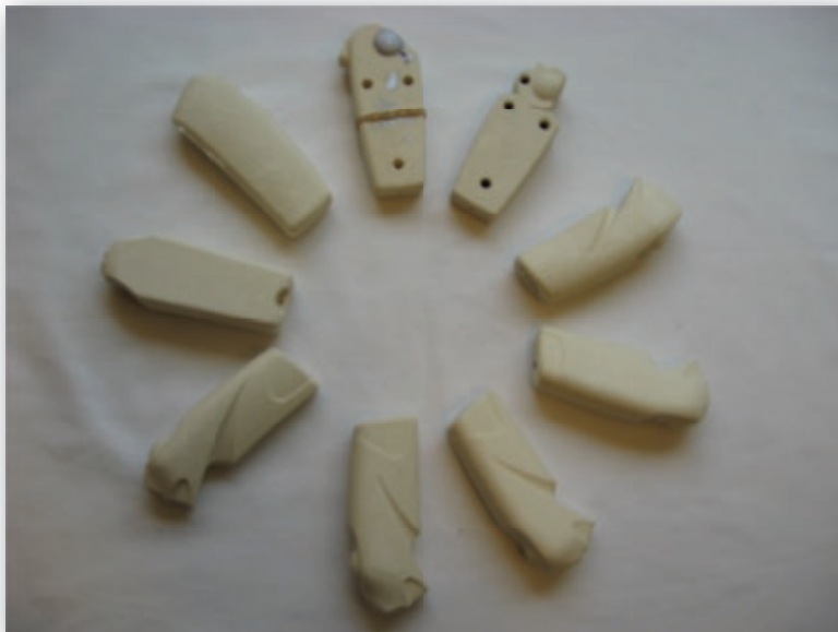
Figure 10. 3D printing and other rapid prototyping techniques can help the product team quickly create and test large numbers of forms with small variations
