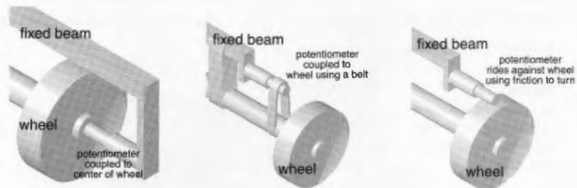
Figure 9.9 Three different methods for coupling a potentiometer to a wheel.
