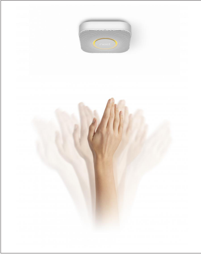
Figure 1-9. Nest’s wave-to-hush feature allowed users to silence the smoke alarm; it was deactivated when it was realized that users might wave their arms in panic during a real fire and unintentionally deactivate the alarm (image: Nest).
