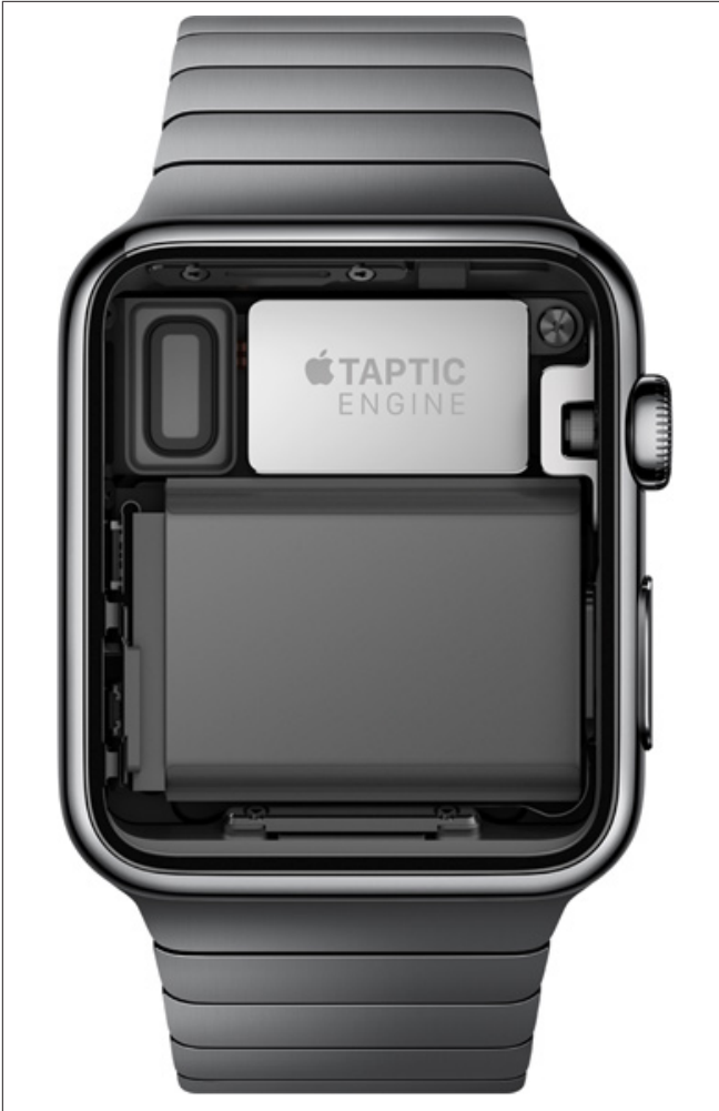
Figure 1-11. The Taptic Engine is a linear actuator inside the Apple Watch that can tap the user on the wrist (image: Apple).
