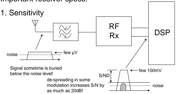
Sensitivity is the lowest input signal level (in dBm) detectable by the receiver while still meeting the min acceptable BER at the DSP detector
