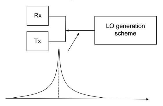
The integrated phase noise under the LO skirt translated into phase jitter in the time domain. The LO phase noise is important for both S/N and EVM.
