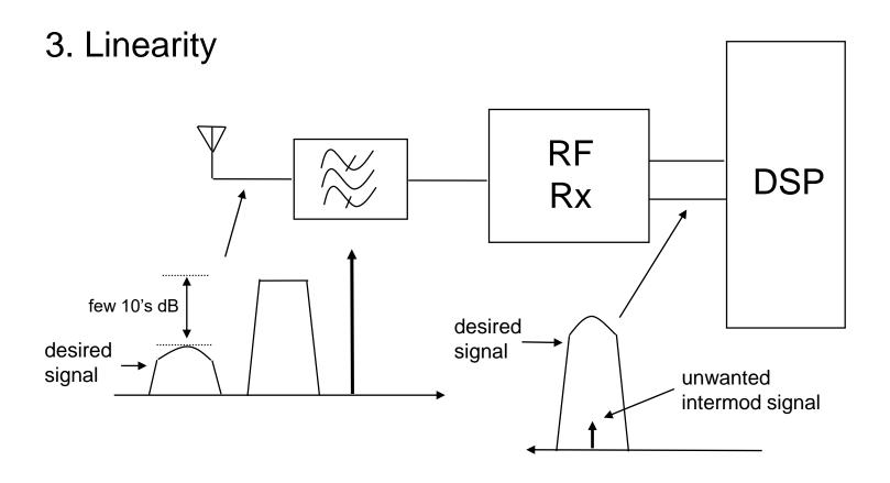
Rx Linearity is defined in terms of 3<sup>rd</sup> and 2<sup>nd</sup> order distortion/intermod levels at the receiver output calculated from the overall acceptable noise+distortion at the detector
