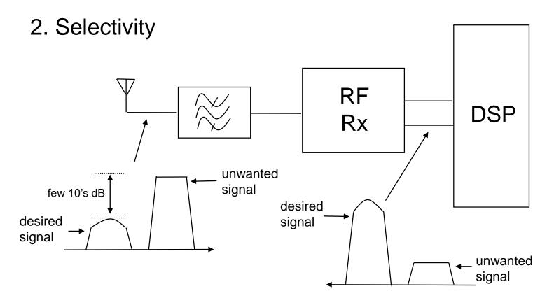
Selectivity is the level ratio of desired signal to all other "unwanted" interferers in dB (integrated over the signal bandwidth). The interferer is sometimes as high as 60dB above the desired signal!
