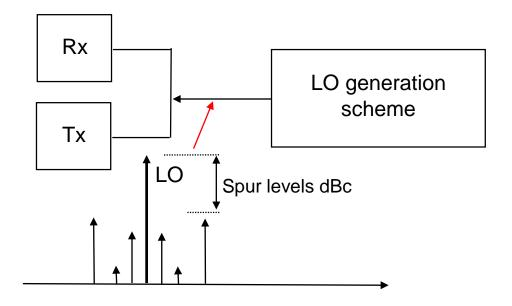
The spectral purity of the LO generation scheme is defined as how many dB down are the worst case spurs relative to the desired LO signal
