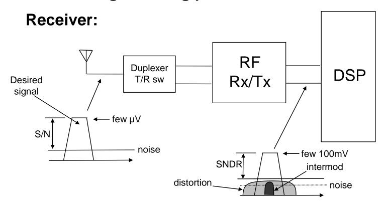
Receiver output SNDR not to be lower that the required level for min BER under ALL conditions for a given standard/modulation
