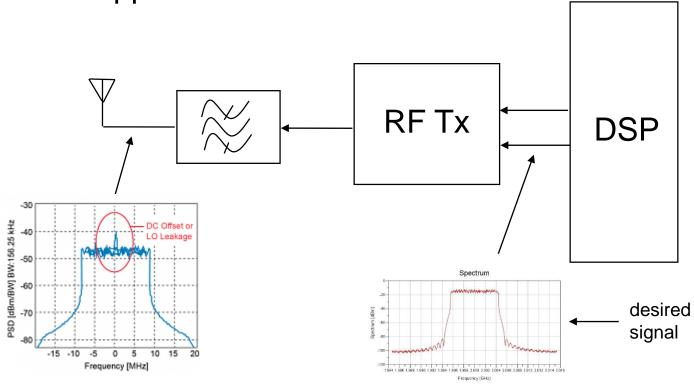
standard regulates a certain carrier suppression requirement. The ratio between signal level and carrier in dB (over specific RBW) is the carrier suppression
