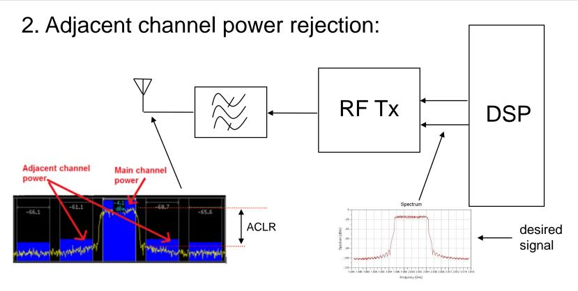
Due to finite transmitter linearity and noise, some of the unwanted transmitted power falls on the adjacent channel frequency band. The ratio between the transmitted power of the desired band over that of the adjacent cannel is the Adjacent Channel Level Rejection (ACLR)
