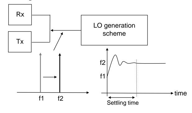
The LO generation is required to settle within few kHz within specified number of µs so as not to lose any Rx packet or corrupt the Tx spectral mask.
