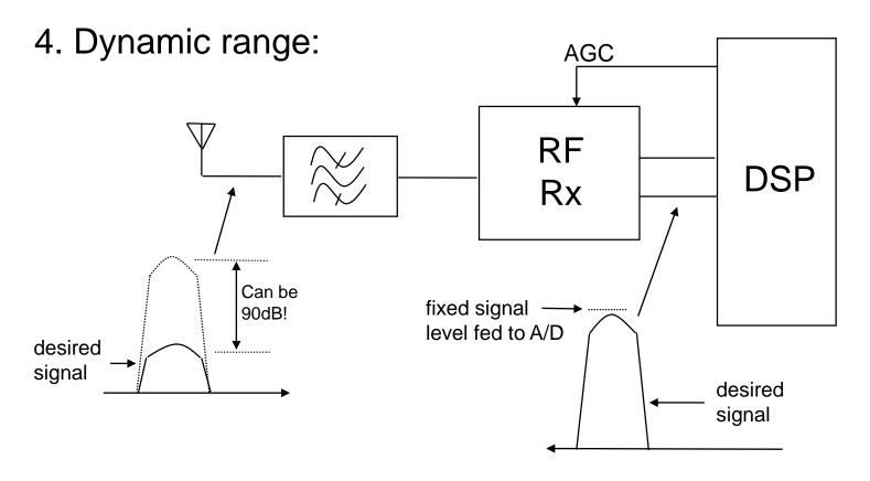
Receiver must sustain a fixed signal level to DSP A/D despite the variation of the desired signal level at the antenna by as much as 90dB (dynamic range). The level is set by the A/D dynamic range
