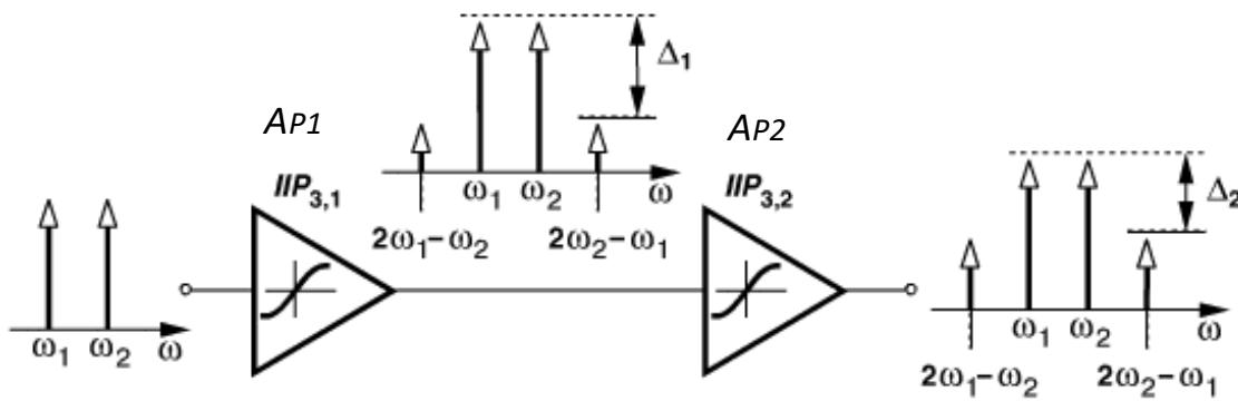
$$\frac{1}{IIP3_{total}} = \frac{1}{IIP3_1} + \frac{AP_1}{IIP3_2} + \frac{AP_1 AP_2}{IIP3_3} + \dots$$
