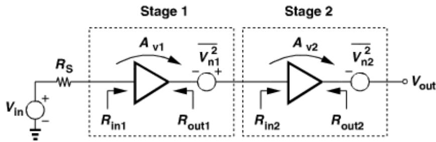
$$A_0 = \frac{V_{out}}{V_{in}} = \frac{R_{in1}}{R_{in1} + R_S} A_{v1} \frac{R_{in2}}{R_{in2} + R_{out1}} A_{v2}$$
