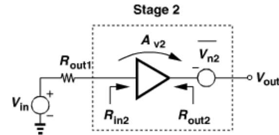
$$NF_2 = 1 + \frac{\overline{V_{n2}^2}}{\frac{R_{in2}^2}{(R_{in2} + R_{out1})^2} A_{v2}^2} \frac{1}{4kTR_{out1}}.$$
