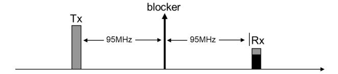
The Tx leakage is -27dBm after duplexer. The B1 blocker level is -15dBm at antenna. In class, we calculated the receiver IIP3 requirement due to this arrangement for a diplexer rejection of 30dB at B1 (result came as -7.9dBm without margin). Let us assume you found another diplexer that provides 31dB rejection to blocker at B1 (1dB better than the one we used in class), how
