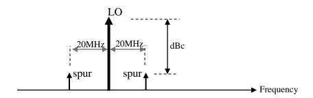
With the adjacent channel n+4 (or 20MHz away from desired signal) level of -40dBm, calculate the relative spur level in dBc (relative to the main LO) so that the folded n+4 signal in-band due to the PLL spur has a <u>negligible</u> impact on the receiver sensitivity of -117dBm.
