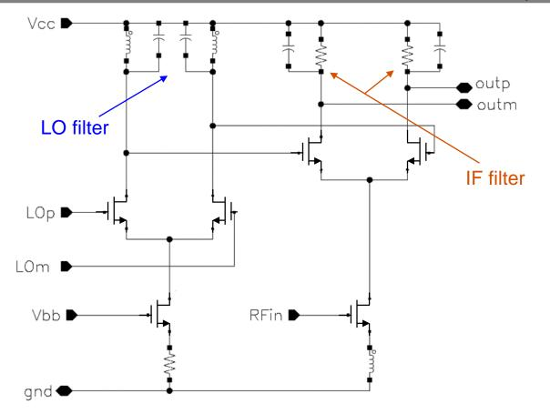
To reduce the sensitivity to LO noise, a bandpass filter is placed at the LO port to filter out any LO noise at the IF band, as shown above. It is important here to note that the effect of the LO noise can be highly suppressed if the LO signal is an ideal square wave with zero rise and fall time. This can be shown as follows
