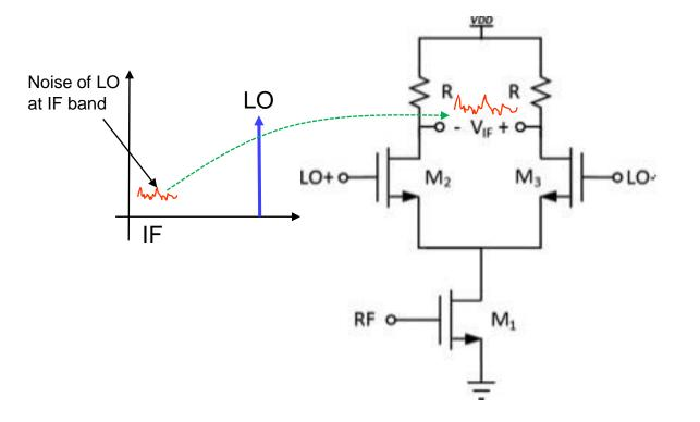
The above circuit is an example of a single-balanced mixer. The diff-pair M2-M3 behave like a differential amplifier to the LO signal. M1 acts in this case as a current source in the absence of the RF signal. With this arrangement, any signal, or noise, occupying the IF band at the LO port will get amplified and transferred right to the mixer output on top of desired IF signal causing significant degradation to the mixer NF.
