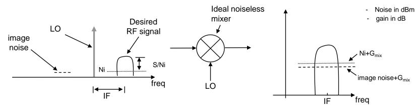
Because of the image problem, a receive mixer down converts both desired and the image bands to IF frequency. This means folding the noise at the image frequency on top of the desired band at IF.
