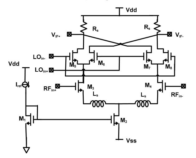
Current-source M2 can be replaced by either a choke or an LC-tank for better headroom and better noise
