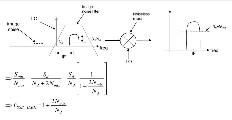
As seen from the IEEE SSB equation, if the mixer is noiseless, the mixer SSB NF is actually 0dB, the spirit behind the new definition.
