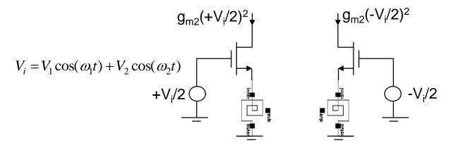
Any mismatch in the Gm stage half circuit (due to circuit components or layout) results in a finite differential IM2 at the output. This low frequency IM2 gets upconverted by the LO when it reaches the quad and so won't appear at the IF output of the mixer. However, any DC offset in the LO quad will result in this IM2 differential component to appear at the mixer output. This can be verified as follows.
