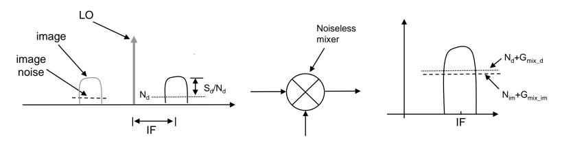
The double-side band NF definition assumes that the image band contains both noise and an image signal identical to the desired band signal. This definition is useful in direct-conversion receiver where the image is the signal itself. Therefore, one can write:
