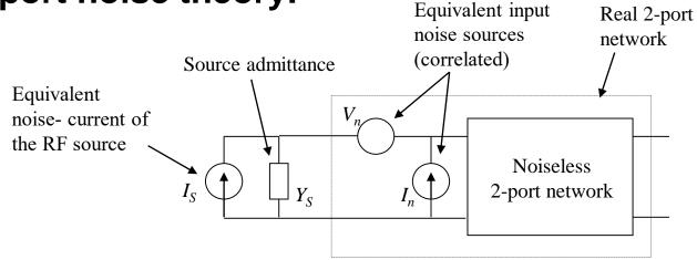
The equivalent input noise sources,  $V_n$  and  $I_n$ , are partially correlated.  $I_n$ , can be decomposed into two components: one is proportional to  $V_n$  through some correlation admittance,  $Y_C$ , and the other component,  $I_u$ , is uncorrelated with  $V_n$ . This can be expressed as:
