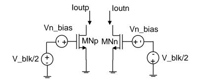
Taking only the terms due to second order nonlinearity to calculate the noise desense:
