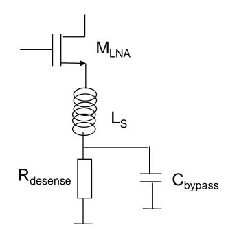
Isolating the bias noise is not enough to prevent noise desensitization due to a blocker. This is because the low frequency noise generated within the LNA core itself mixes with the blocker causing the desense. To improve this, one must do the following:
