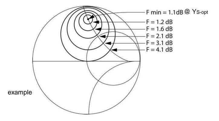
The NF contours (circles) are centered around YS-opt and plots the NF in the admittance domain as a function of YS. This shall give the designer an idea on how to trade-off NF vs power match. Please note that any changes to the circuit (active or passive) changes Ys-opt and NFmin values. We will discuss later in class how to manipulate circuit to get simultaneous NFmin and power match
