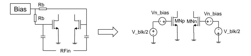
The bias noise is represented as a common-mode noise in series with the gate of each side of the differential input transistors. The blocker is placed differentially with a half circuit representation as shown above.
