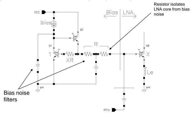
Another source of low frequency noise is that generated within the LNA core itself. This low frequency noise usually gets amplified by the relatively large DC gain of LNAs. Therefore, reducing the low-frequency LNA gain results in improving the LNA noise desense.
