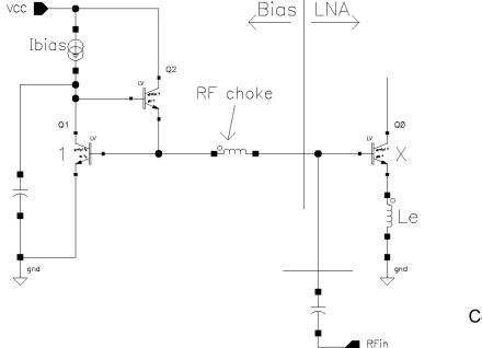
The bias network has also an impact on the LNA IP3. It is has been shown that for good IP3, the LNA impedance looking into the LNA input much be very low at the tone spacing frequency of the IP3 two tone test [5]. This can be achieved by an off-chip series resonance network (L\_trap, C\_trap) that acts like a short at the tone spacing frequency (for example 10MHz for the two tone frequency of 2150, 2160MHz).
