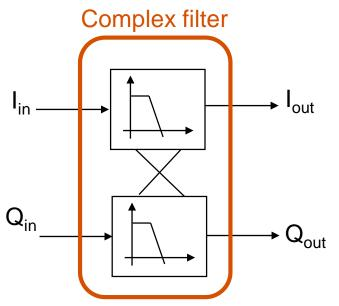
There is nothing complex about complex filters. They are called "complex" because they have two orthogonal signals (I and Q) as inputs and each of their orthogonal (complex) outputs depends on both complex inputs. Mathematically, it is easier to represent orthogonal signals as complex signals (I + jQ). This representation makes math a lot easier. For example, if
