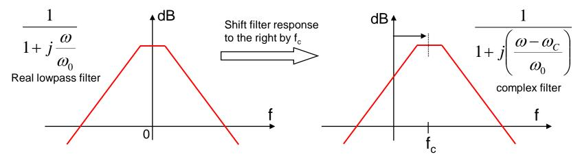
Complex filters in a sense show a simple way of realizing bandpass filters. However, there is a real difference between the two. Real bandpass filter does not discriminate against image.
