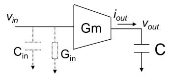
The finite input conductance, as well as parasitic input capacitance, of the Gm cell can be modeled as a finite  $G_{in}$  and  $C_{in}$  in parallel with the input. Since the filter realization is a cascade of biquads and integrators, the input of a Gm cell loads the output of the other resulting in the same impact on the transfer function as  $G_{out}$ , and  $C_{out}$ .
