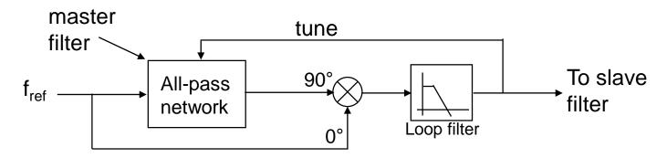
The allpass network uses the same Gm/C or opamp-RC blocks in the main filter to construct the following function:
