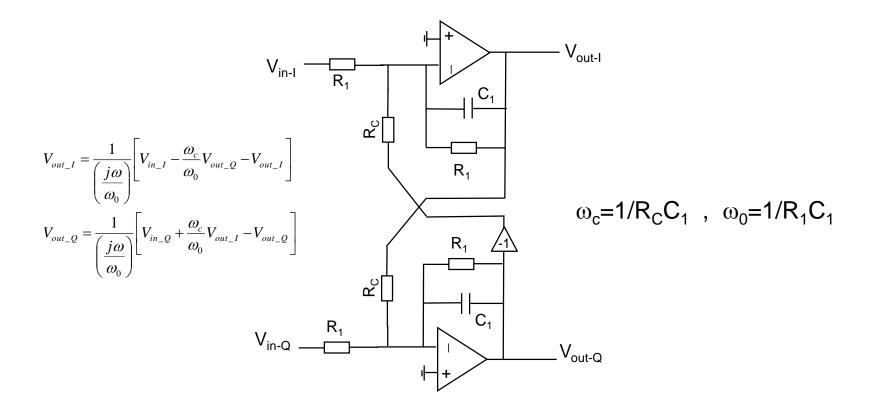
Note that the I/Q coupling resistor (R<sub>C</sub>) decreases as the frequency shift  $\omega_c$  increases. With  $\omega_c = 0$  (no shift, R<sub>C</sub>= $\infty$ ) the complex filter collapses to two independent I/Q real first-order lowpass filters.
