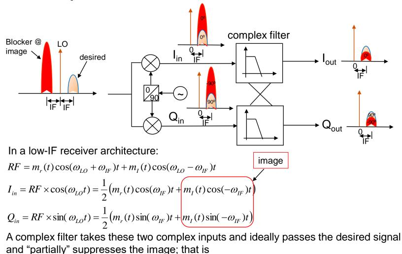
$$I_{out} = \frac{1}{2} \left( m_r(t) \cos(\omega_{IF}) t + \delta m_I(t) \cos(-\omega_{IF}) t \right) \quad \text{; and} \quad Q_{out} = \frac{1}{2} \left( m_r(t) \sin(\omega_{IF}) t + \delta m_I(t) \sin(-\omega_{IF}) t \right)$$
