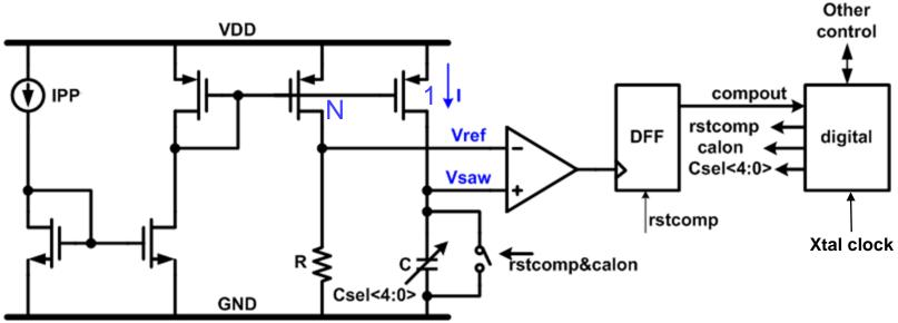
$$V_{ref} = N.I.R = N \frac{V_{BG}}{R_{ref}}R = costant$$
