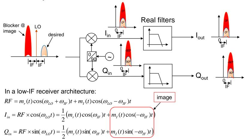
As seen the image blocker (can be 10'sdB higher than desired) falls on top of desired signal. Real low-pass filter does nothing to this because blocker already fell in-band. The ADC then needs to have enough dynamic range to handle this combined power of blocker+desired so digital baseband can perform image suppression.
