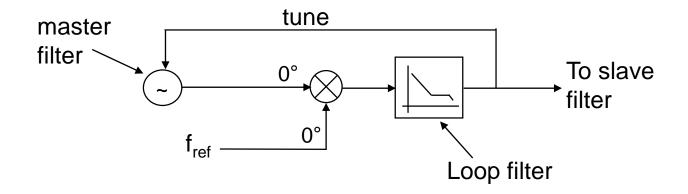
The above architecture is a simple phase-locked loop. The VCO is constructed using the same Gm/C or opamp-RC cells used in the main filter. This is a relaxation-type VCO whose oscillation frequency  $\omega_0$  is dependent on Gm/C or RC. The loop ensures that the VCO frequency is always equal to the precision reference frequency fref which is usually coming from a xtal oscillator.
