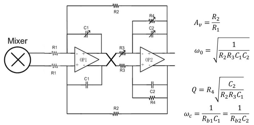
This is a biquad (real low pass filter). First you chose circuit parameters based on noise, linearity and signal BW. Next step is to design the cross coupled resistors between I and Q filters to create a complex filter as shown next
