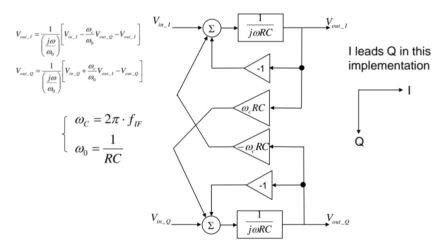
Note that when  $\omega_c$  is zero, the diagram collapses to a simple "real" first order lowpass filter for each I and Q.
