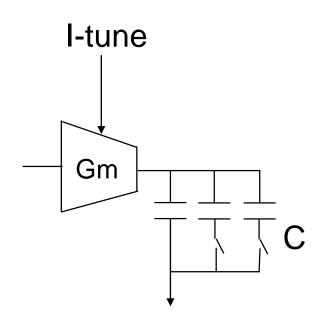
• Digital tuning adds to area overhead. It also introduces parasitic poles/zero to the overall TF.
