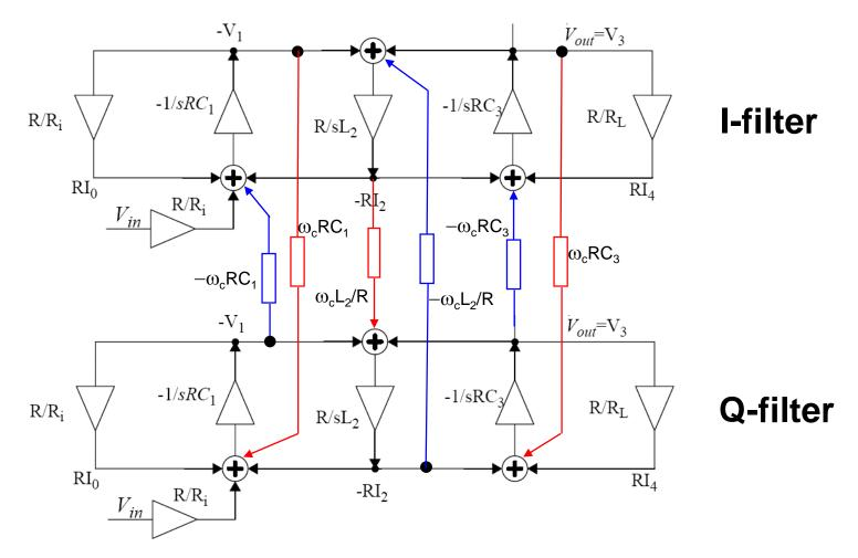
Only 3 integrators per filter are needed to implement this complex bandpass filter as compared to 6 integrators per filter for real bandpass filter implementation!
