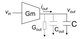
The finite output conductance of the Gm cell can be modeled as a finite  $G_{out}$  in parallel with the integrating cap. Similarly, the parasitic output capacitance of the Gm cell appears is parallel with the integration capacitor. This means the ideally lossless integrator becomes a bit lossy with the following transfer function:
