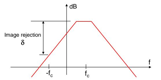
Note that the image rejection level,  $\delta$ , is set by the filter order (3<sup>rd</sup>, 5<sup>th</sup>, etc.), filter function (Butterworth, Chebyshev, etc) and the frequency shift, fc. It is also set by the I/Q input magnitude and phase matching. If achieved image rejection  $\delta$  is sufficient for SNR, you need only either I or Q signal (not both) to send to digital baseband.
