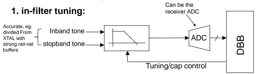
Two equal tones are injected into the filter, one at a time. The first tone is at a passband frequency, while the other is at a stopband frequency with known filter rejection value. The two tones are measured at the filter output with the aid of the ADC. Digital baseband adjusts the filter tuning code until the exact rejection value is met. This assumes the filter is only process dependent, but temperature and Vdd independent. Retuning is needed when temperature drifts
