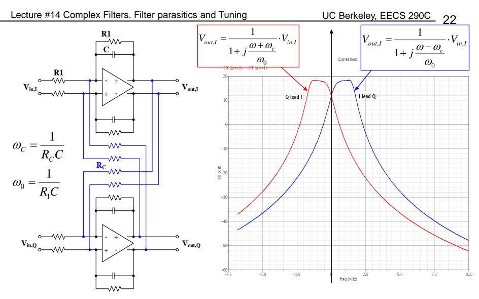
Note that you can decide to favor upper mix or lower mix in this low-IF receiver (meaning positive vs negative frequencies) by changing the sign of the cross-coupled resistor voltages (I leads Q or Q leads I). The not flat passband is due to finite opamp GBW Copyright© Dr. Osama Shana'a
