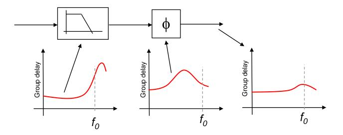
Allpass networks are used for filter group delay equalization. This is because they only impact the phase (and hence group delay) of the filter and not the filter amplitude.
