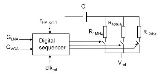
• the use of a switchable highpass corner controlled by a digital sequencer each time an "event" of LNA gain switch of VGA switch occurs.
