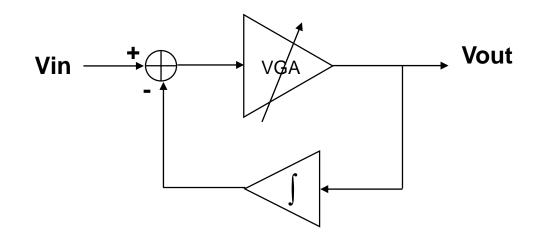
a servo loop is just an integrator put in the feedback loop between the VGA output and its input as shown. The new input-output relation can be derived as
