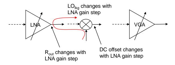
• the LNA output impedance changes slightly with LNA gain switch. This modifies a bit the reflected component of the LO leakage, resulting in a small change of DC offset at the VGA input. This results in a nasty DC offset kick at the VGA output, especially at max gain, before the servo loop has the time to correct for it.
