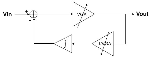
The idea is to insert a block in the feedback loop whose function is the inverse of the VGA forward gain. In other words, this block has the inverse AGC slope of the forward path VGA. The new transfer function is then:
