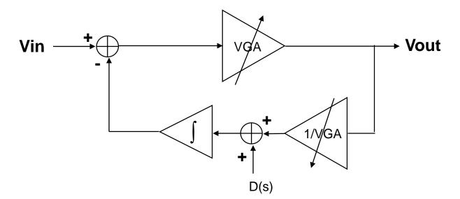
Let us the investigate the impact of the 1/VGA nonlinearity on the overall VGA distortion. The distortion due to the 1/VGA block can be injected into the loop as shown above. This distortion then reaches the VGA output through the following transfer function:
