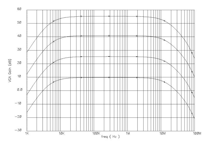
With modified servo loop scheme, <10% variation of high-pass corner over 60dB AGC is obtained
