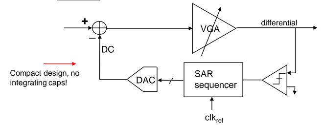
• a comparator detects the differential output offset and its sign. Based on the offset sign, the comparator triggers a successive approximation register sequencer to start counting up or down
