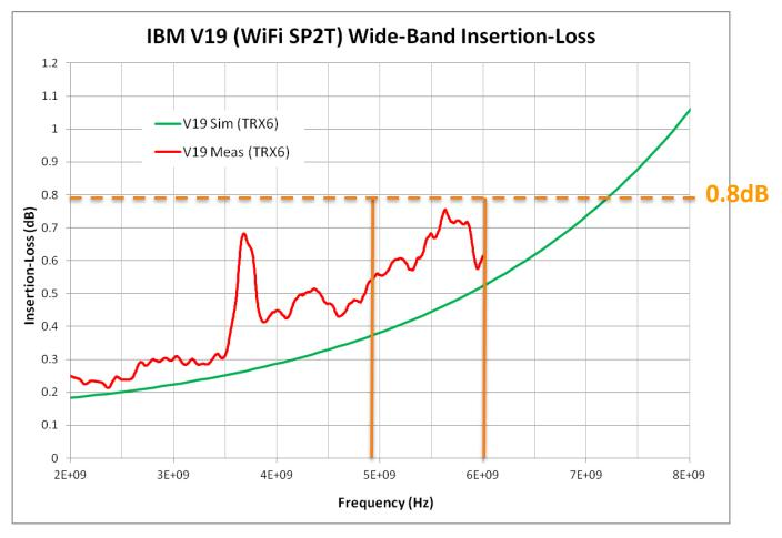
Remarkable insertion loss of 0.55dB is achieved at WiFi 5GHz. The switch is designed for broadband RF. If it is optimized for 5.5GHz, a better IL can be achieved. This switch has P1dB>+35dBm
