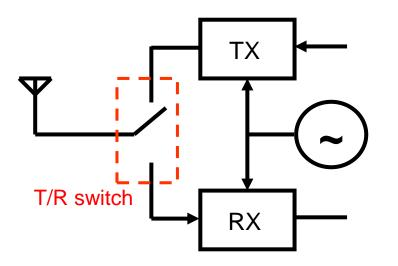
In TDD system, both Tx and Rx share the same antenna via a T/R switch. They also share the same RF band, so they alternate in time (Time Division) with either Tx is ON and is connected to antenna, or Rx is ON and is connected to antenna (but not both ON at the same time during normal operation).
