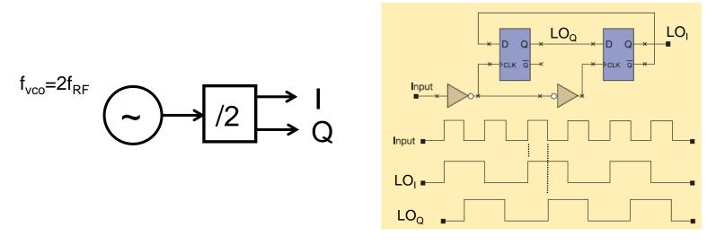
A disadvantage of this scheme is that there is an upper limit on the frequency it can operate at. Up to this moment, reliable low power VCOs with integrated tank run at about 12GHz or lower. This means the maximum RF frequency this scheme can serve is below 6GHz.
