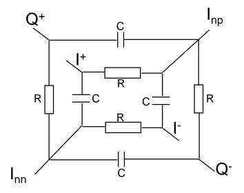
The problem with polyphase filters is that they are lossy. Therefore, a significant amount of current is needed to drive them. Furthermore, the phase matching expected worsen with higher frequency. A typical I/Q phase matching is 3° for 3-sigma.
