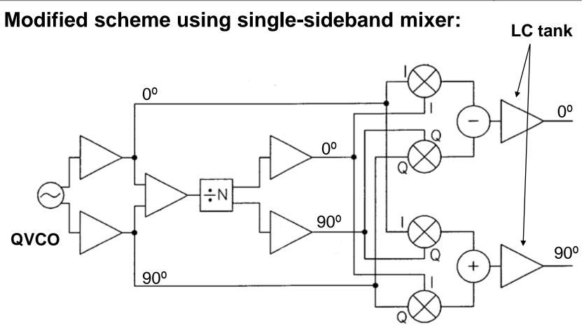
The single-sideband mixer provides additional 20~30dB rejection to the 1/3LO component in addition to the 20dB rejection provided by the LC tank at the output. The disadvantage of this scheme is you need either a quadrature VCO or generate a quadrature VCO signal from VCO output via poly-phase network
