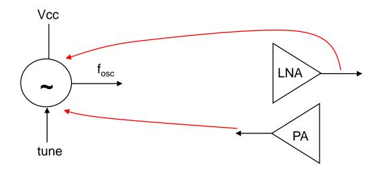
integrating the VCO with PA, and/or LNA makes it prone to pulling. This is due to finite isolation on-chip between these blocks. The VCO pulling is the disturbance of the oscillation frequency due to presence of large signals on-chip. The LNA/PA coupling to VCO can be via:
