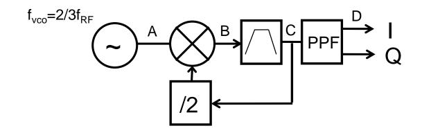
$$B = \frac{C}{2} \times A \Rightarrow f_B = \frac{f_C}{2} + f_A \text{ OR } f_B = f_A - \frac{f_C}{2}$$
