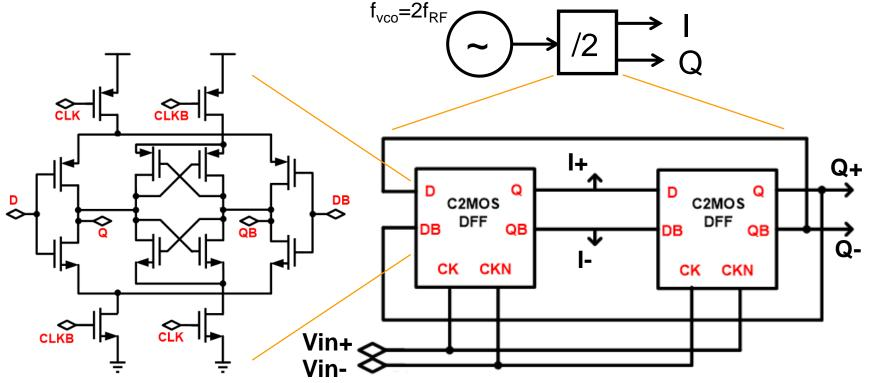
A master-slave flip-flop architecture is the most common for a divide-by-2 LO generation scheme. The flip flop is implemented using CMOS logic circuit that fits the speed of a given technology (CML, C2MOS, etc.). Device sizing (hence current) is set by divider speed requirement (max input frequency) and I/Q phase matching requirement. Please note that the transition of the divider output is set by the transition (zero-crossing) of the input clock
