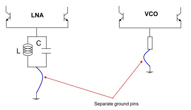
Note that if an exposed paddle package is used, a dedicated ground pin has only 10dB isolation to the paddle at 2GHz. Therefore, a lateral isolation (separation) between ground pins is needed, in addition to having orthogonal orientation to minimize bond-wire coupling.
