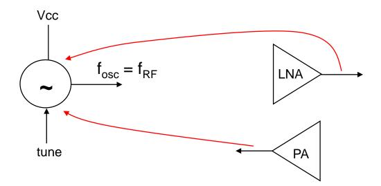
In this scheme, VCO, LNA and PA are all operating at the same frequency. Let us assume that the VCO loop (with both LNA and PA off) has a single frequency solution ( $A\cos\omega_0 t$ ) that satisfies the criteria of oscillation. That is:
