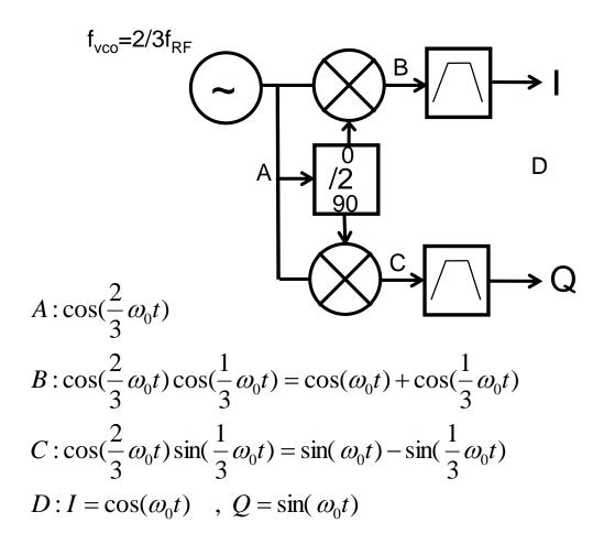
Note that only the tank rejection attenuates the unwanted mixer side band at  $(1/3)\omega_0$ , which is around ~20dB typical (not sufficient)
