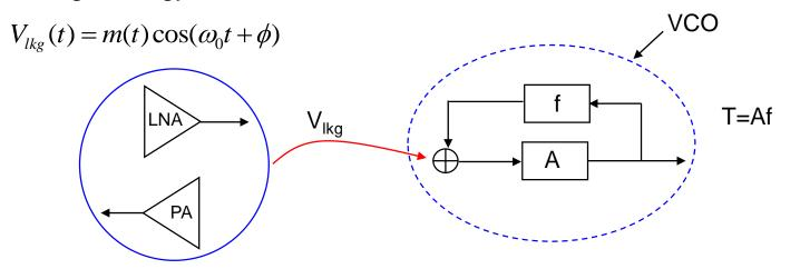
The leakage energy will disturb the equilibrium of the feedback circuit of the VCO. The disturbance can be viewed as modification of both magnitude and phase around the VCO loop. As a result, there will be a new "solution" of the loop that satisfies the criteria of oscillation. If the leakage energy is only a pure tone of the same frequency as of the VCO (m(t)=0 and  $\phi$  is constant), then this results only in a phase shift of the oscillation signal.
