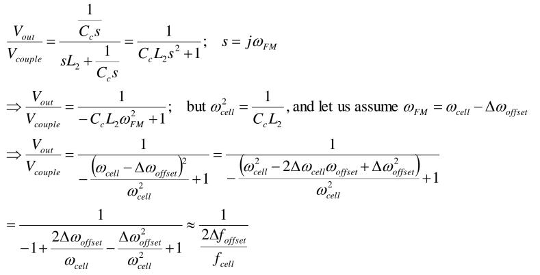
the "gain" by which  $V_{\text{couple}}$  gets to the VCO tank collapses to
