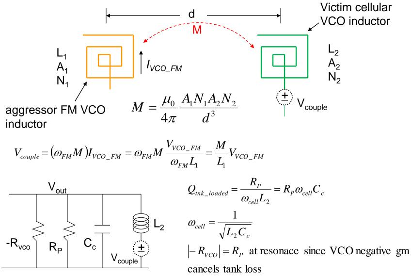
Cell VCO tank R-L-C model at resonance
